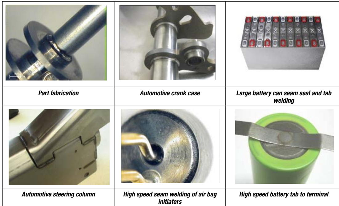
Figure 47 – Examples of CW laser welding
