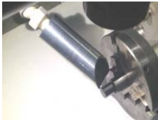
Figure 49 – Tube promoting laminar flow of argon
